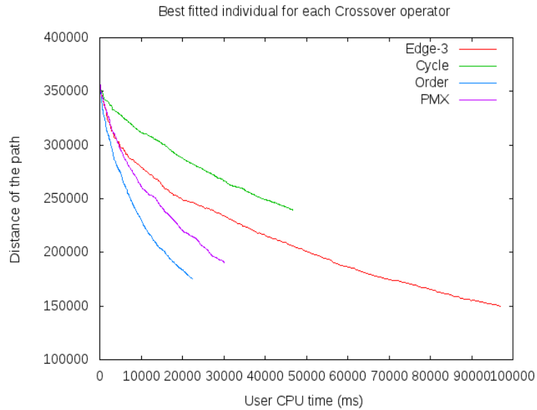
Figure 8: Comparison of Crossover Operators on a 1000 cities TSP, x axe is user-cpu time
